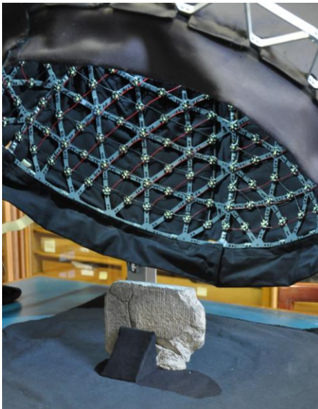
Fig. 1. Recording of a large tablet with the PLD.
